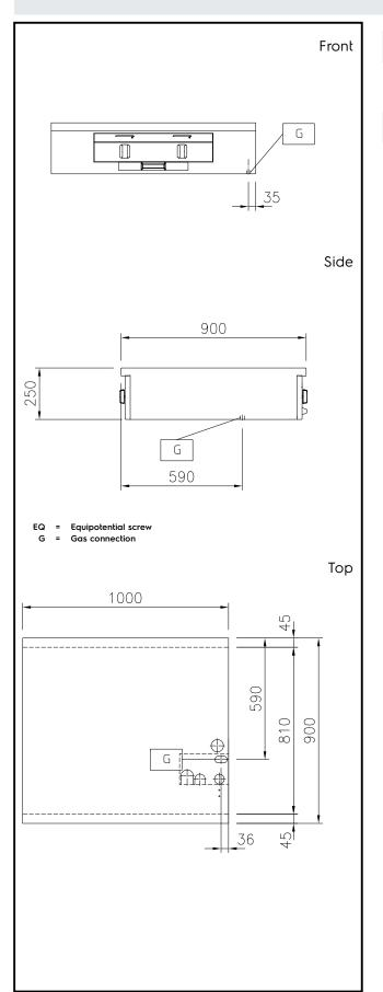
Gas Gas Power: 34 kW Gas Type Option: Gas Inlet: 1/2" **Key Information:** External dimensions, Width: 1000 mm External dimensions, Depth: 900 mm External dimensions, Height: 250 mm Net weight: 82 kg Configuration: Two-Side Operated;Top Front Burners Power: 8.5 - 8.5 kW **Back Burners Power:** 8.5 - 8.5 kW **Back Burners Dimension -**Ø 70 Ø 70 mm Front Burners Dimension -
